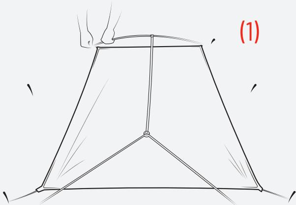
3. Assemble all of the poles and insert the pole tips into the four corner eyelets on both the inner and groundsheet. The poles should bend upwards when pitching the last two sections to create the tent shape. [Fig 1]
