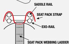
FIG 2: CROSS SECTION OF SEAT CLAMP
