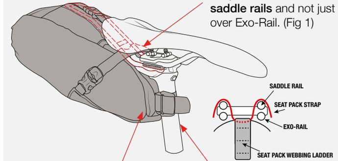
FIG 1: CROSS SECTION OF SEAT CLAMP
