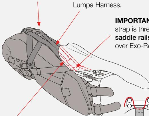
Loop Lumpa strap back around Exo-Rail bar to pull seat pack in tight.
